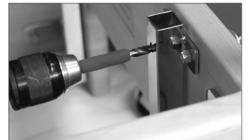
Figure J: Drill through receiver and into Reformer until drill bit hits the mounting plate.
